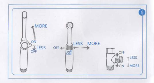
10.Please note that if you feel that the water pressure is too high or too low, you can adjust the water pressure to the strength you want by adjusting the switch at the T-adapter and the sprayer at the same time.
