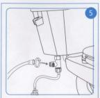
6.Connect the other end of shower hose to the handheld bidet sprayer head. Please be sure to check that the seal ring is safely in place before hand tightening the connection again.
