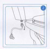
3.Connect the T-adapter valve to the flush tank. Hand tighten the T-adapter valve to the flush tank.
